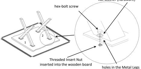
STEP 3: Place the double ended spanner key 13 mm around the screw and rotate it clockwise.
